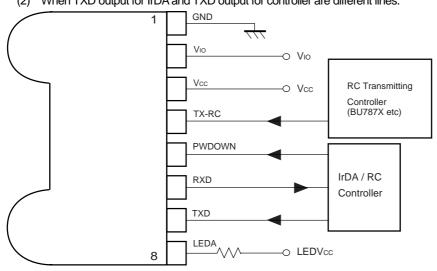
(2) When TXD output for IrDA and TXD output for controller are different lines.
