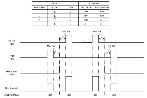
(2-b) RC transmit mode at IrDA receiver power down condition.
